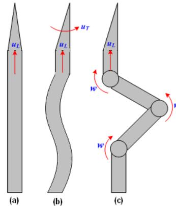
Fig. 1 Different paradigms of needles (a: conventional rigid; b: flexible; c: active)
